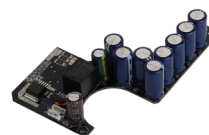
*Failsafe via internal super capacitor
