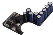
*Failsafe via internal super capacitor
