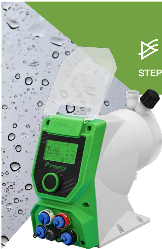
The PRISMA diaphragm and stepper motor metering pump is designed for applications requiring high precision dosing volumes and reliable repeatability. Thanks to the microprocessor controlled stepper motor and excellent pitch resolution of 1: 4800, the entire stroke and suction cycle is controlled with maximum precision. Maximum steps frequency: 180 st/m.
