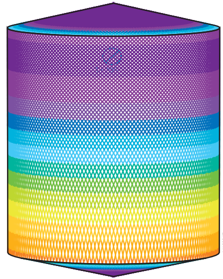
D4.6m H5.5m, Toftejorg TJ40G, 4 x ø7.3 mm, Time = 16 min., Water consumption = 5600 l
