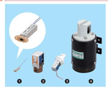
In the case of a conventional (e.g. N.C. - Normally Closed) solenoid valve, continuous energisation is required to maintain open status. The latching solenoid doesn't require a power supply for the purpose of maintaining open status through the utilisation of a permanent magnet. Suitable for applications where the power consumption and the effect of temperature on a fluid is a concern.
